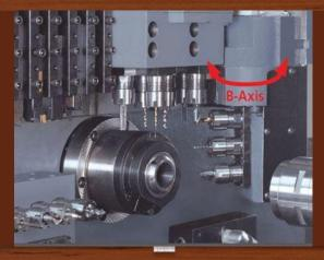
The Eurotech SwissTurn Zeit is an 8 axis Swiss type auto lathe with fully programmable B-axis for cutting on the main and sub spindle; it accepts any major brand guide bushing and collet; easy conversion from guide bushing to non guide bushing; plus many additional features that come standard:
