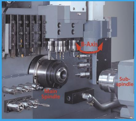
Eurotech SwissTurn ZEIT Swiss-Type CNC -9-axis and up to 42 mm, with 2 Y-axes, B-axis, C-axis and sub-spindle.
