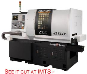
The Zeit-CSL42 → showing gang-style turning tools, rotary cutters, B-axis capabilities, and subspindle with end working tools.
