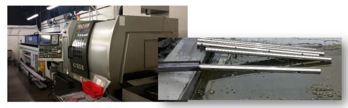
"The Eurotech Zeit machine was our first machine with the B-axis capability, which allows us to machine the parts in one operation instead of two. This of course is a huge savings in time and improves part quality," noted Pat Hundley, President
